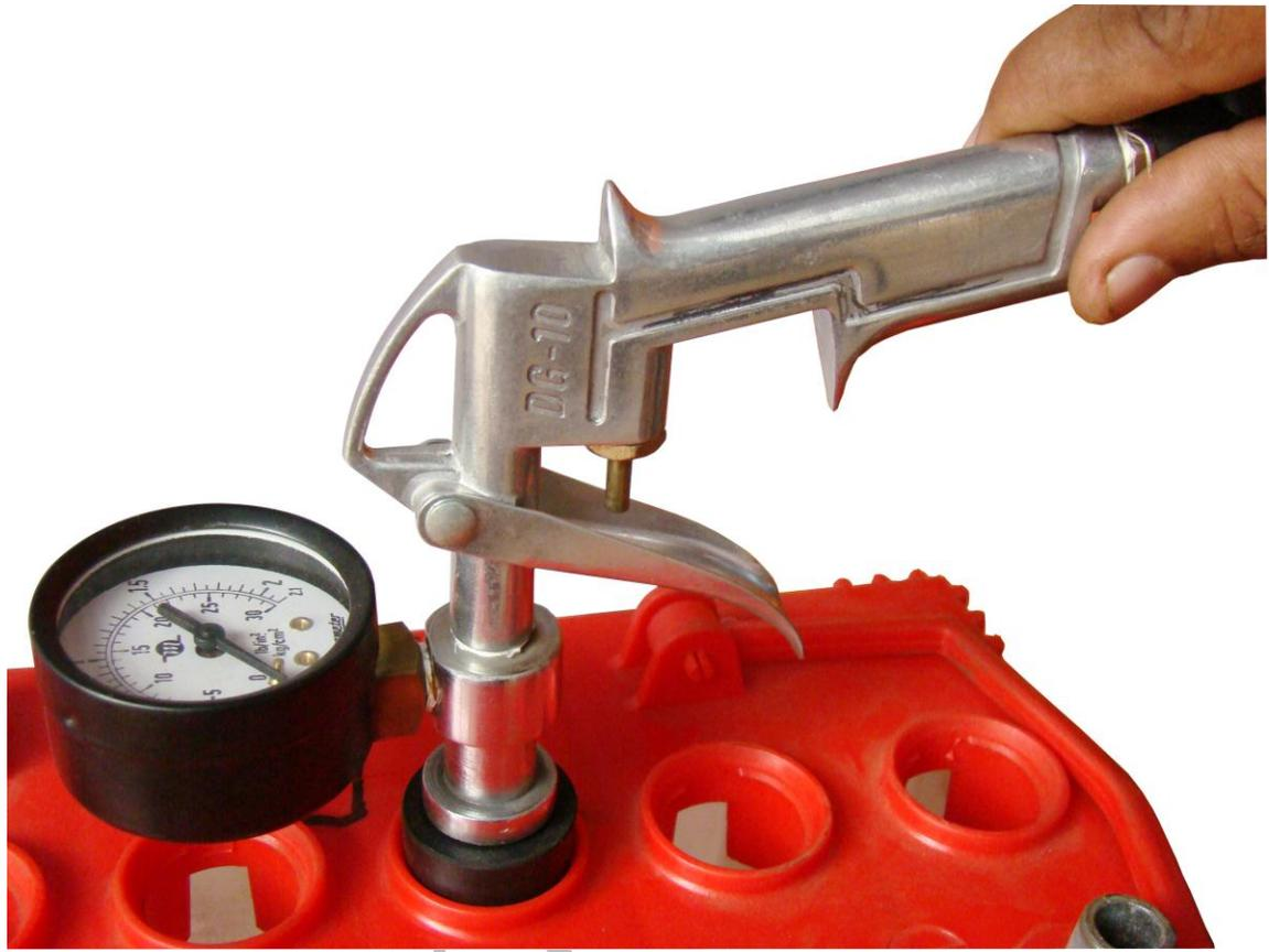
d. There may be leakage cell to cell leakage but not from sealing, it can be from welded L connection at partition.
