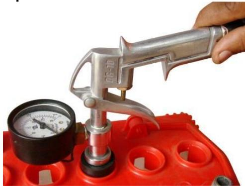
**O3. SHORT CIRCUIT TESTER (ONE CELL IN ONE GO):**
