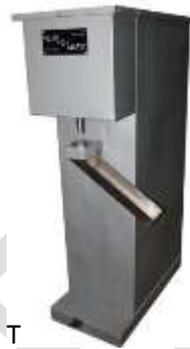
This machine is fitted with interchangeable die. This die can be changed by pick & place technique. This machine is pneumatically operated and initiated by Pedal Valve. Cut Lid is placed on die and machine is operated by pressing foot on valve. Top punch presses Pole out of Lid. This can be seen in the video. Now, Lid will be without Lead parts. Of course, Lead parts will be having bit of Plastic in which it is molded. This Plastic can be ignored.
