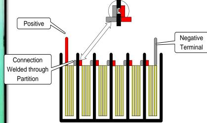
For Inter Cell Welding Through the PARTITIONS OF BATTERY
